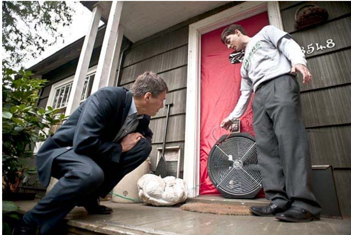
Vancouver Mayor Gregor Robertson views the Embers blower-door test in action (CARMINE MARINELLI, QMI AGENCY)
