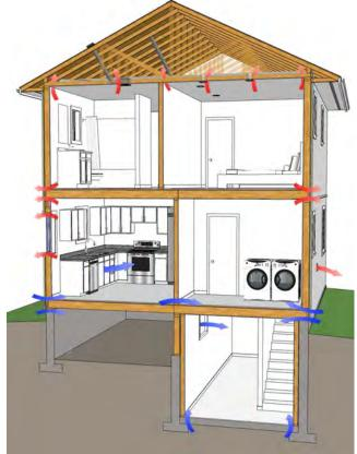
part basement and crawlspace with a ventilated attic roof. Arrows show typical air leakage locations to review and
