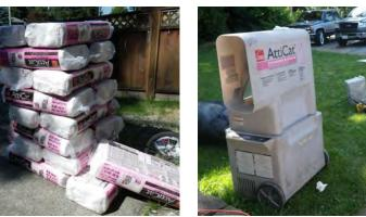
Blown-in insulation prior to installation and blowing machine.
