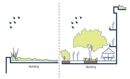
Figure 6a. Extensive Green Roof
