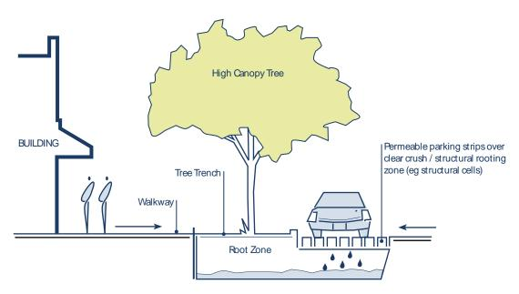
Figure 5. Permeable Paving
