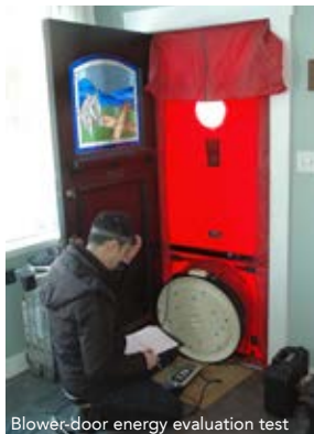
Blower-door energy evaluation test
