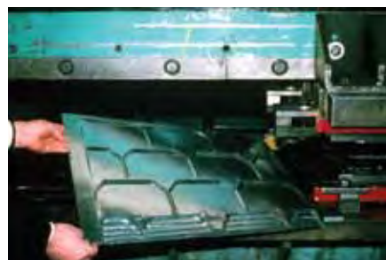
A surviving pressed metal shingle was used as a prototype for manufacturing replacement shingles when restoring the main house at the Motherwell Homestead near Abernathy, SK. In Restoration, repairs or replacements of extensively deteriorated or missing parts of features are done in kind, and are based on physical, documentary and oral evidence.
